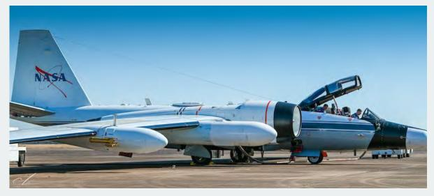
Scientists from CSL, along with collaborators from the Global Monitoring Lab, NASA, and several universities traveled to Ellington Field in Houston, Texas this past February for a round of engineering test flights on NASA's WB-57 high altitude aircraft. The team was testing out new and modified atmospheric instruments designed to measure trace gases and aerosols high up in the stratosphere.
