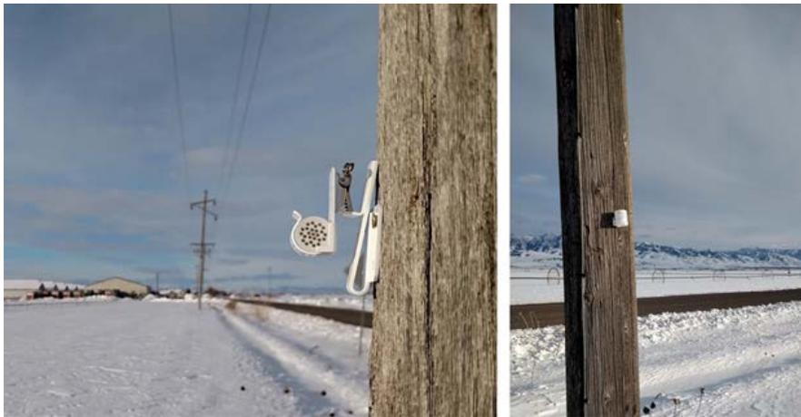
Figure 2.10 Passive ammonia sampler as deployed at the rural Lewiston (Cache Valley) sample location – without (left) and with the wind/precipitation cap (right).
